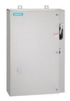
Non-reversing motor starter Size 2 Three phase full voltage Solid-state overload relay OLRelay amp range 13-52a 24VAC 50-60HZ coil Combination type 60Amp non-fused disconnect Encl NEMA type 4X 316 S-steel Water/dust tight non-corrosive Extra-wide enclosure
