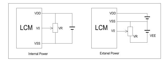
V<sub>DD~</sub>V<sub>0</sub>: LCD Driving voltage
