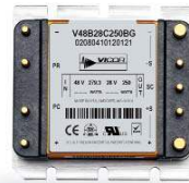
Mini example: V48B28C250BG 48 Vin, Mini, 28 Vout @ 250 W, long RoHS pins, slotted baseplate
