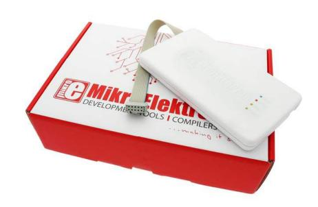
mikroProg<sup>TM</sup> for MSP432 is a fast and reliable USB programmer and hardware debugger. This mikroProg supports the SimpleLink<sup>TM</sup> MSP432<sup>TM</sup> microcontroller family from **Texas** Instruments.
