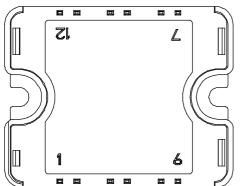
All multiple inputs and outputs must be shorted together 1/2; 5/6; 7/8; 9/10; 11/12
