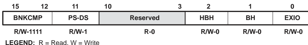
Figure 6. Bank-Switching Control Register (BSCR), MMR Address 0029h
