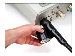
3.5 Starting 1" (25 mm) below the previous layer of vinyl tape, wrap the entire cable and connection section with three continuous half-lapped layers of <sup>3</sup>/<sub>4</sub>" (19 mm) wide vinyl tape.
