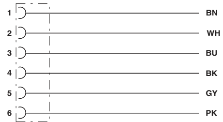
Contact assignment of M8 socket
