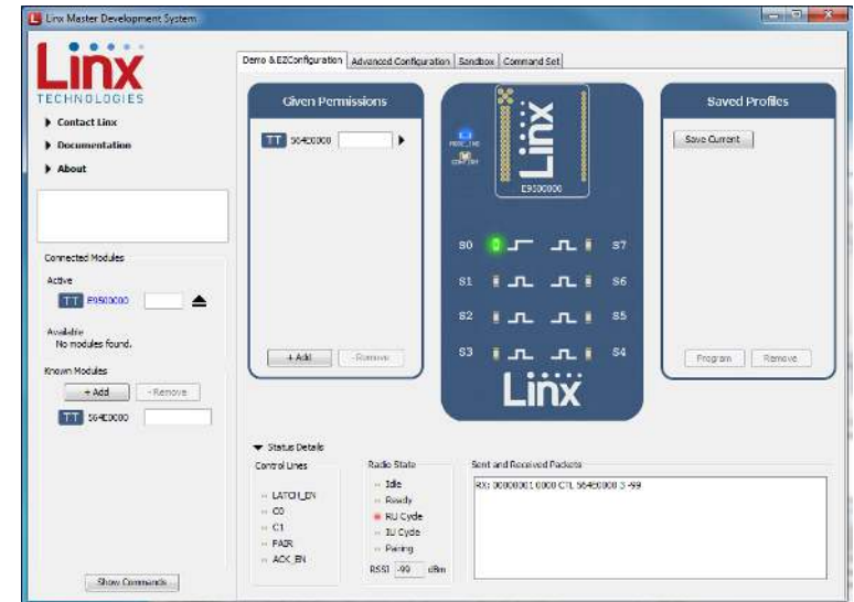
Figure 31: The Master Development System Software Receiving Module
