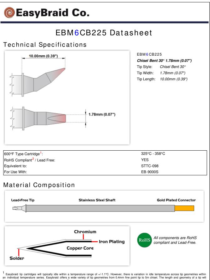
an individual temperature series. Easybraid oriers a wide variety of tip geometries from 0.4mm fine point tip to 5m chisel. The length and geometry of a tip will have an influence on the tip idle temperature. To accurately measure idle temperature it will depend greatly on the measurement method, technique and equipment used. Two different methods or the use of alternative equipment will produce different test results.
