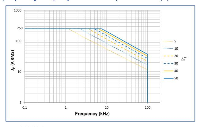
Primary current in A RMS is sine wave.
