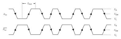
For all allowed capacitive range, recommended load resistor  $R_i$  = 100 Ohm. Logical 1 is coding on a rising edge on  $D_{\text{out}}$ .
