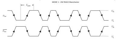
For all allowed capacitive range,  $\it R_{\rm L}$  can be 100 Ohm. Logical 1 is coding on a rising edge on  $D_{\text{out}}$ .
