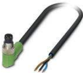
Sensor/Actuator cable, 3-position, PVC, Black RAL 9005, Plug angled M8, on Free cable end, Cable length: 10 m
