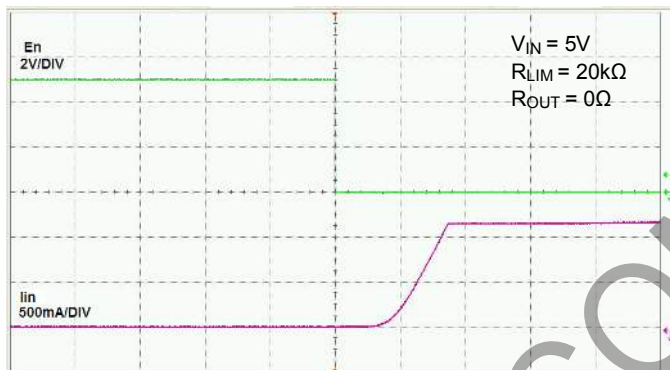
500μs/div Figure 5. Device Enabled into Short-Circuit
