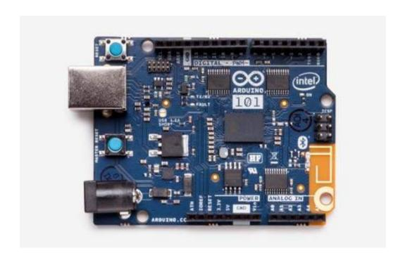
**Arduino 101** combine the ease-of-use of the classic boards with the latest technologies. The board recognises gestures, and features a six-axis accelerometer and gyroscope. Control your projects with your phone over Bluetooth connectivity!
