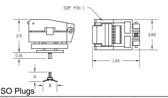
SO Plugs are required to connect this adapter to the prototype. They are available separately. The two most common plugs are shown in the following chart. Other SO-Plugs will also mate with this adapter, contact us if you want assistance matching plugs to this adapter.
