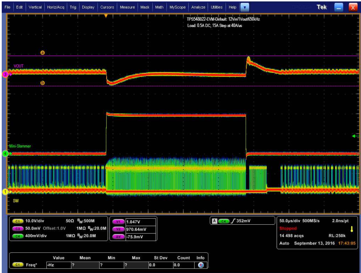
Figure 9-4. Transient Response of 1-V Output at 12 V IN , Transient is 0.5 A to 15.5 A, the Step is 15 A at 40 A/μs
