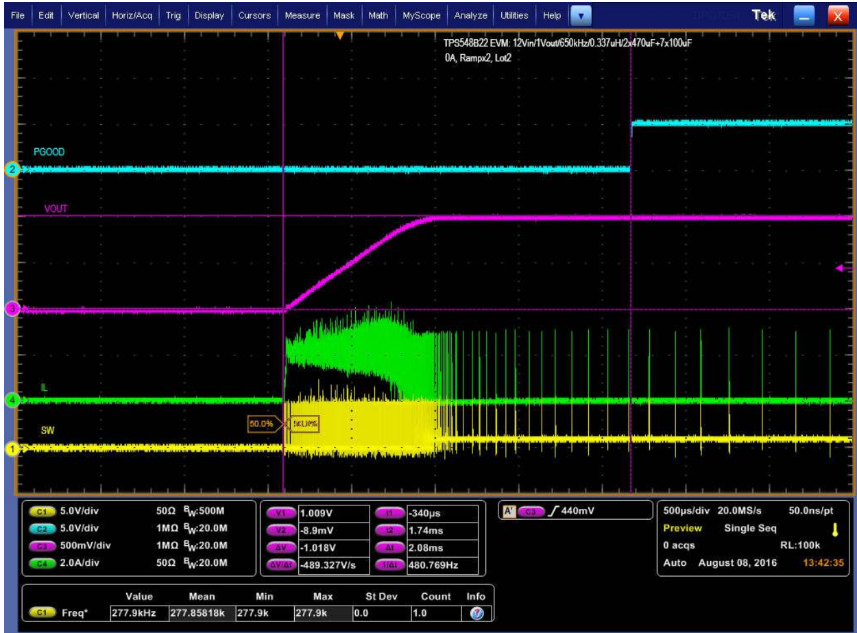
Figure 9-7. Start up from Control, 1-V Output at 12 V IN , 0-A Output
