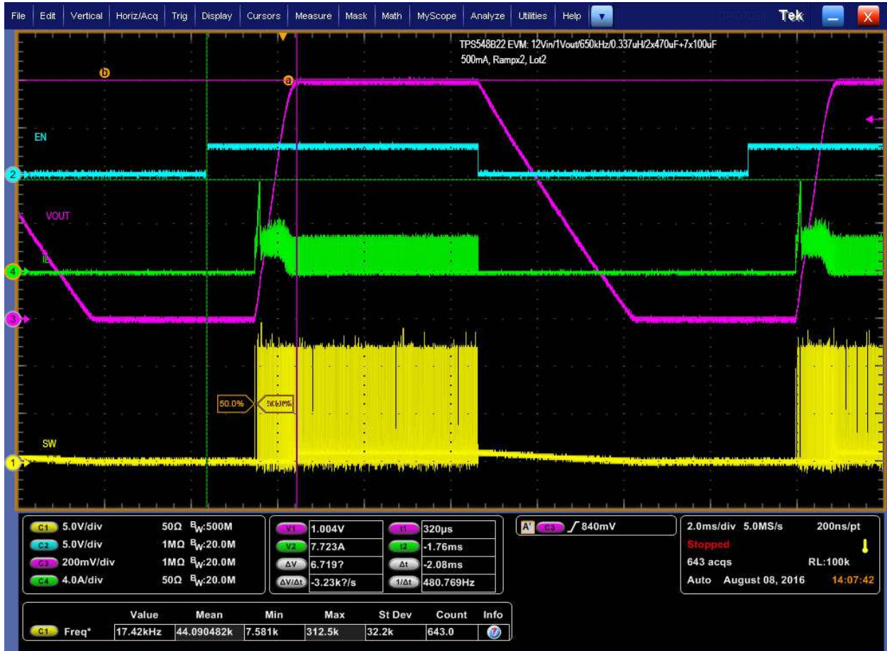
Figure 9-9. Output Voltage Start-up and Shutdown, 1-V Output at 1 2V IN , 0.5-A Output
