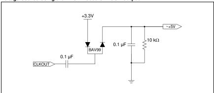
Most bus switches have extremely low-current requirements, so despite the limited current sourcing capability of CLKOUT, it can potentially be used to both generate ~5V required for the bus switches and still be used as a clock source for other circuitry in the application.
