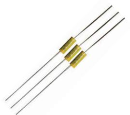
Type WMC axial-leaded polyester film/foil capacitors are ideal for automatic insertion in printed circuit boards. It is an ultraminiature version of Type WMF and the sections of these non-inductive capacitors are constructed with extended foil, polyester film, with tinned copper-clad steel leads.
