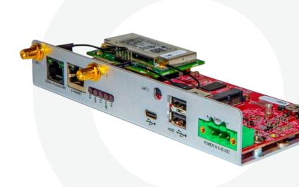
**Full REST API on-board and a Linux-based runtime environment** – making it easy to create and configure custom applications.
