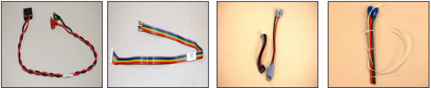
Figures 4-7: From left to right: Power supply to driver board cable, Signal cable, Driver board to LED cable, Thermistor cable
