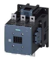
power contactor, AC-3 400 A, 200 kW / 400 V AC (50-60 Hz) / DC operation 23-26 V AC/DC auxiliary contacts 2 NO + 2 NC 3-pole, frame size S12 busbar connections drive: conventional screw terminal
