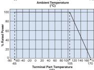
For resistors operated at a terminal part temperature of described for each size or above, a power rating shall be derated in accordance with the derating curve.
