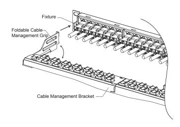
5. Fix the solid cables to the cable fixture hole using cable ties.
