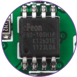
Figure 11-1: Flash memory module
