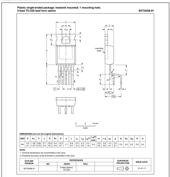
Fig.4. SOT263B package<sup>1</sup> leadform 263B-01, pin 3 connected to mounting base.
