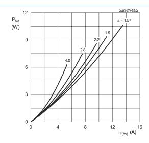
a = form factor =  $I_{F(RMS)}$  /  $I_{F(AV)}$ V<sub>o</sub> = 0.532 V; R<sub>s</sub> = 0.0077  $\Omega$
