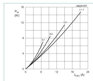
$\begin{aligned} I_{F(AV)} &= I_{F(RMS)} \times \sqrt{\delta} \\ V_o &= 0.532 \text{ V; } R_s = 0.0077 \text{ } \Omega \end{aligned}$
