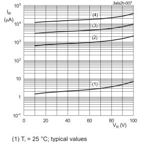
(2)  $T_j = 100 \,^{\circ}\text{C}$ ; typical values (3)  $T_j = 125 \,^{\circ}\text{C}$ ; typical values
