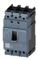
circuit breaker 3VA5 UL frame 125 breaking capacity class M 35kA @ 480 V 3-pole, line protection TM210, FTFM, In=40A overload protection Ir=40A fixed short-circuit protection Ii=10 x In UL489 SB (naval), 50 deg. cel. nut keeper kit on both sides
