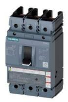
circuit breaker 3VA5 UL frame 250 breaking capacity class C 100kA @ 480V 3-pole, line protection TM230, FTAM, In=80A overload protection Ir=80A fixed short-circuit protection li=5...10 x In without connection
