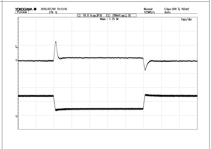
Figure 4: Dynamic response to load step 25%~75% with 0.1A/uS slew rate at 110/220Vac TOP: V_{out} , 200mV/div, BOTTOM: I_{out} , 10A/div, 1mS/div
