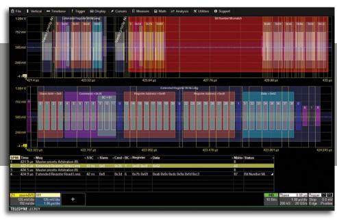
The MIPI System Power Management Interface (SPMI) decoder provides a fast and easy way to understand and correlate SPMI bus traffic to DC power rails and power management IC (PMIC) operations in mobile, handheld, and battery-powered embedded systems.
