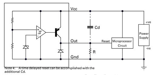
$$T_{DY} = RCd \left[ In \left( \frac{1}{V_{TH}} \right) - In \left( \frac{1}{1 - \frac{V_{SAT}}{V_{in}}} \right) \right]$$
