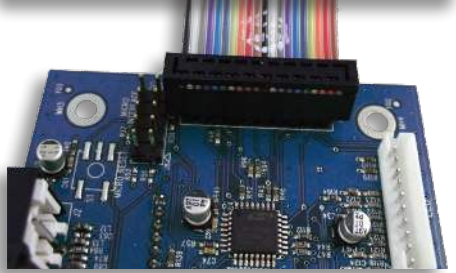
▲ DSP Interface Header connected to CRD-USBMASTER-DC-Z daughter card connected via JP1 ribbon cable enables real-time control of the DSP parameters shown in the DSP Composer .CPA signal flow file
