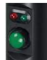
Two leds (red and green) that indicate the locked and unlocked statuses.
