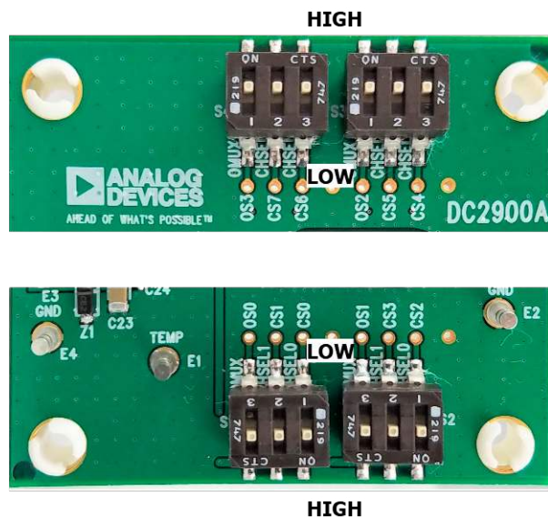
Figure 3. DC2900 Switch Positions for High and Low
