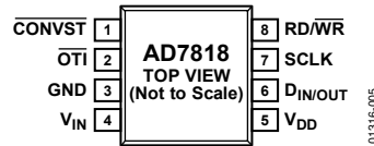
Figure 5. AD7818 Pin Configuration
