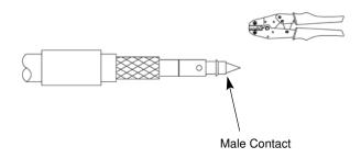
4. Press sub-assembly into body, until contact clicks into place, and ensure that the knurled ferrule is inserted between the dielectric and braid.
