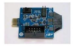
**1.1.2. Si4010 Socketed Key Fob Development Board (P/N MSC-DKPE1)** Socketed (both SOIC and MSOP) key fob board with SMA connector.
