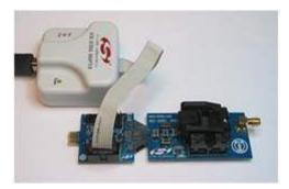
This setup is suitable for downloading, running, and debugging the program in RAM or burning the program in the NVM and running it. The antenna or measuring instrument can be connected through an SMA connector. Since sockets on board allow use of unsoldered ICs, this is the ideal scenario for burning the NVM memory of Si4010.
