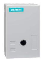
Non-reversing NEMA contactor, Size 1, Three phase full voltage, Contactor amp rating 27A, 3 wire (NO aux included), 240V 50Hz / 277V 60Hz coil, Non-combination type, Enclosure NEMA type 1, Indoor general purpose use, Standard width enclosure
