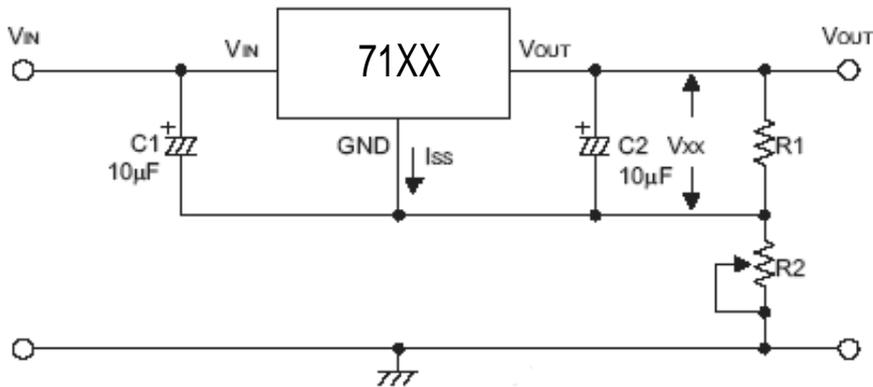
$$V_{OUT} = V_{XX} \left( 1 + \frac{R2}{R1} \right) + I_{SS} \cdot R2$$
