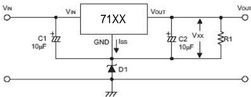
$$V_{OUT} = V_{XX} + V_{D1}$$
