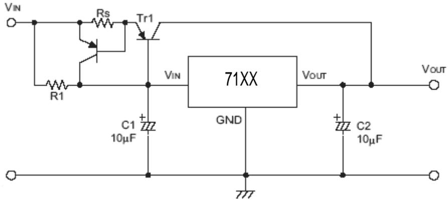
4. Circuit for increasing output voltage (1)
