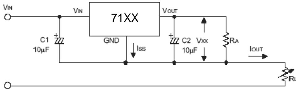
$$I_{OUT} = V_{XX}/R_X + I_{SS}$$
