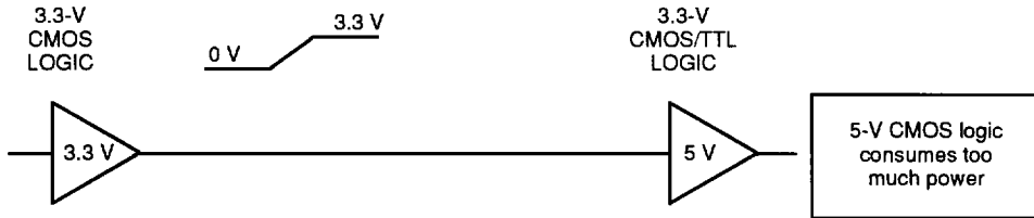
a. 3.3-V Driver to 5-V Input
