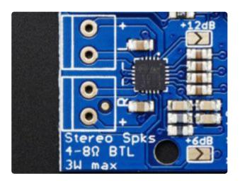
In the bottom left is an amplifier section, this is a stereo 3W amplifier, with bridge-tied load output. It's only meant for driving speakers directly! Do not connect to another amplifier, use the line out for that! Also, you cannot bridge-tie R and L together - if you need only one speaker, leave the unused one disconnected.
