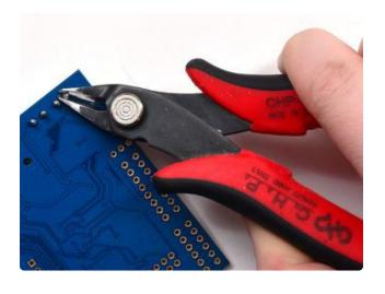
To keep the rightmost speaker pin from bumping into the DC jack you may need to clip it with diagonal cutters
