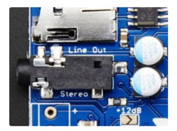
For almost all purposes, the Stereo Line Out 3.5mm jack is what you'll want to get audio out of the shield. It's there on both versions of the shield. The two big silver capacitors on the right are DC blocking caps. This means that the audio is AC-coupled and is safe to use with any amplifier, headphone. etc. Line level is up to about 2V peak-to-peak. If you have a system that really needs 0.7Vpp or less, set the volume on the VS1053 in software.
