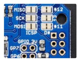
If you're using a Mega or Leonardo Arduino, you'll need to short the jumpers on the top right of the board, and install the 2x3 socket header. This is because those Arduinos use the 2x3 pin header for the hardware-SPI pins and hardware-SPI is required for the high-speed data transfer required by the VS1053 codec. We'll cover that in the Assembly step.
