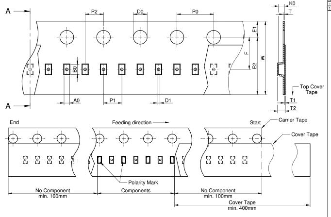
Orientation: Cathode on top Packaging is reffered to the international standard **IEC 60286-3:2013**
