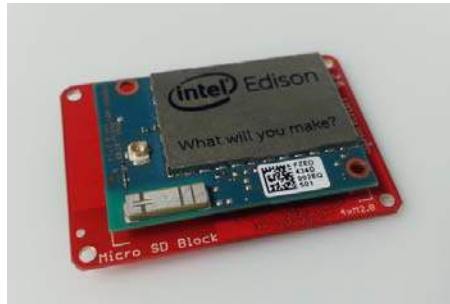
microSD Block Installed
