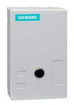
Non-reversing NEMA contactor, Size 0, Three phase full voltage, Contactor amp rating 18A, 3 wire (NO aux included), 220-240/440-480VAC 60Hz coil, Non-combination type, Enclosure NEMA type 1, Indoor general purpose use, Standard width enclosure
