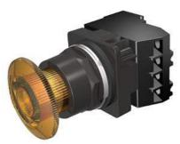
30mm BlackMax, Epoxy Coated Corrosion Resistant Complete Metal Unit Illuminated Twist-to-Release Transformer type, 240V AC Incandescent Lamp Mushroom Head Cap Small 1.79" (45 mm) Plastic Cap, Amber 2 Position Maintained, Twist-to-Release with 1 N.O. - 1 N.C. Heavy Duty Contacts, A600/P600 UL Listed, CSA Certified NEMA 1,3,3R,4,4X,12,13 & Automotive Standards
