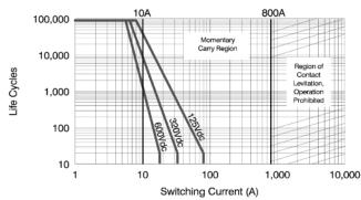
\*Based on extrapolated data. Since each application is unique, user is encouraged to verify rating in actual application. The load terminals should always be connected as follows: Common Contact (A2) positive; Other Contact negative.
