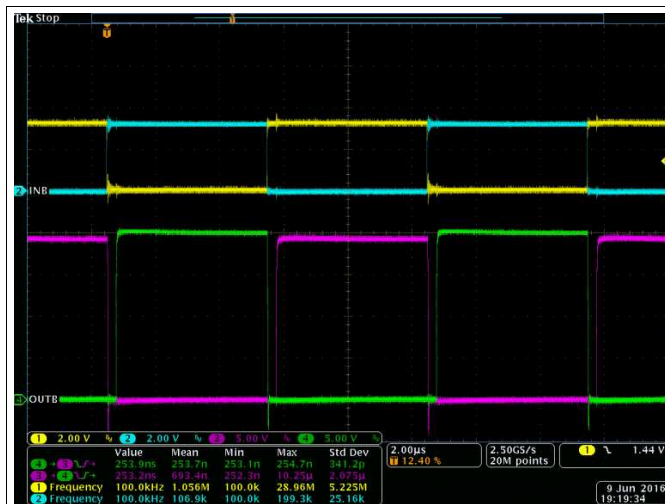
Figure 42. Bench Test Waveform for INA/B and OUTA/B
