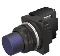
30mm BlackMax, Epoxy Coated Corrosion Resistant Complete Metal Unit Illuminated Indicator Light Full Voltage type, 12V AC/DC Incandescent Lamp, BA9s Glass Lens, Blue UL Listed, CSA Certified NEMA 1,3,3R,4,4X,12,13 & Automotive Standards
