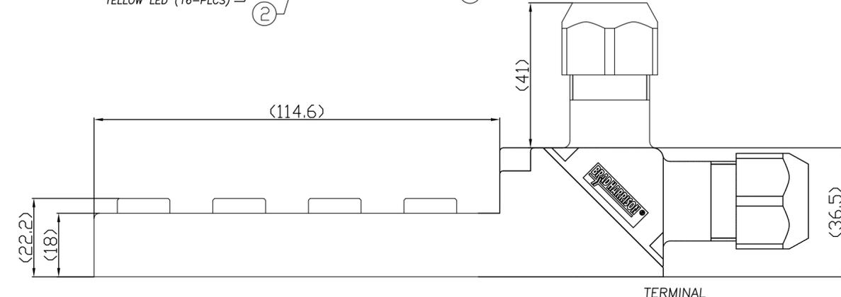
VIEW WITH COVER REMOVED TO SHOW POSITION OF PCB HEADERS
