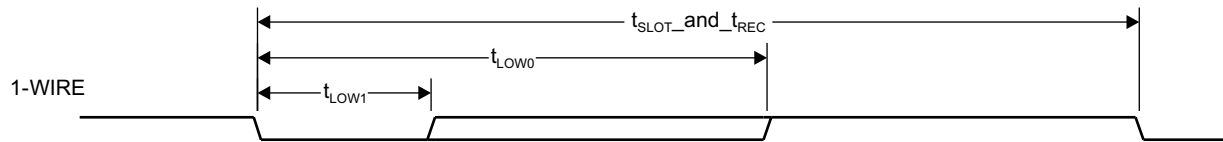
Figure 5-109. 1-Wire Write Bit Timing (Command/Address or Data)
